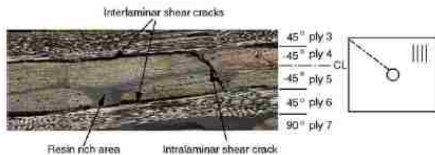
Figure 4. Delamination of composite laminates (Pagano & Schoeppner, 2000)
