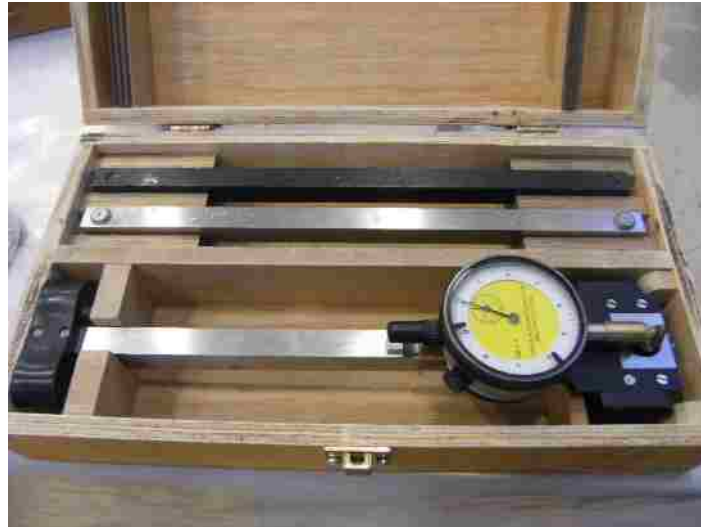
Figure 100. Reference bar and dial gauge used to install and measure DEMEC points
