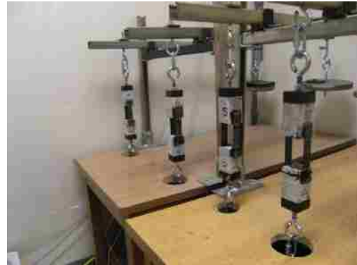
(b) Four creep specimens loaded
