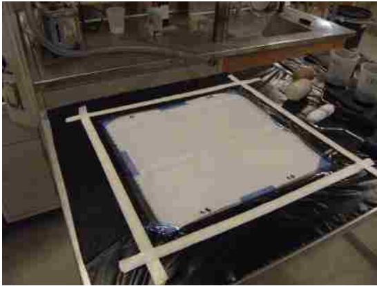
(a) Bottom peel ply is ready for fabric
