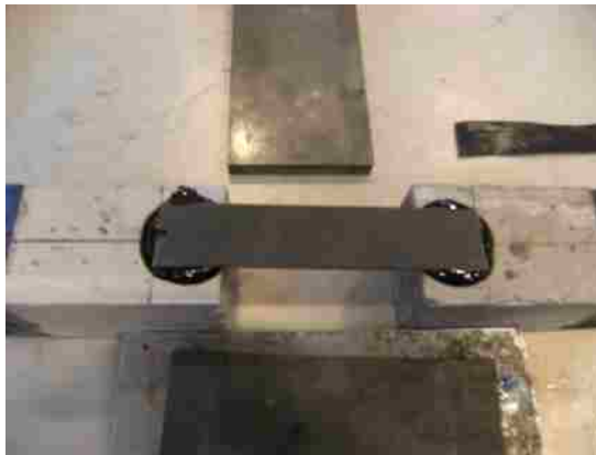
(c) Placement of CFRP sheet on the shear joint
